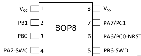
Figure 3-9 SOP8 Pinout1 PY32F002BL15Sx
